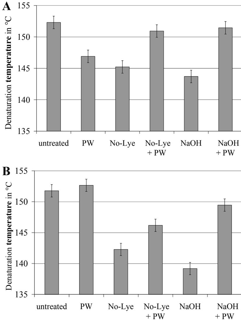
Fig. 38: Denaturation temperature of natural and simulated Afro hair samples
