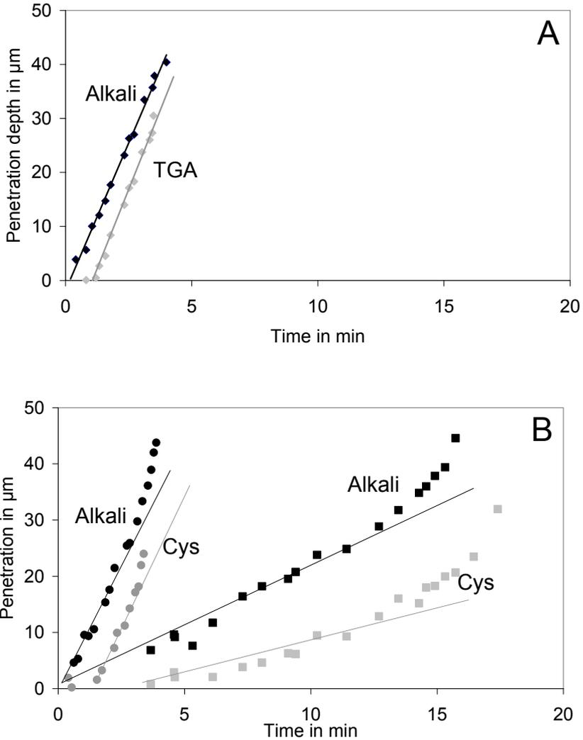
Fig. 71: Penetration depth of inner (alkali) and outer (thiole) penetration front versus time at pH 12.82 + TGA or Cys. While the black dots represent the alkali penetration, the grey dots show the thiole penetration. Mean results are given.
