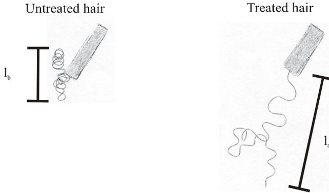
Fig 40: Determination of the effective length of a single hair fiber before ( $l_b$ ) as well as after treatment ( $l_a$ ). The hair is fixed on one end.
