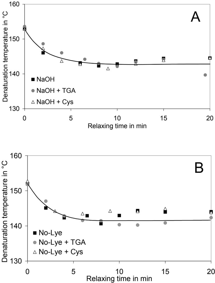
Fig. 54: Denaturation temperature versus relaxing time for different treatments.
