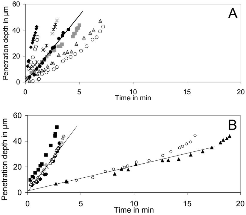
Fig. 70: Penetration depth versus time at different pH.
