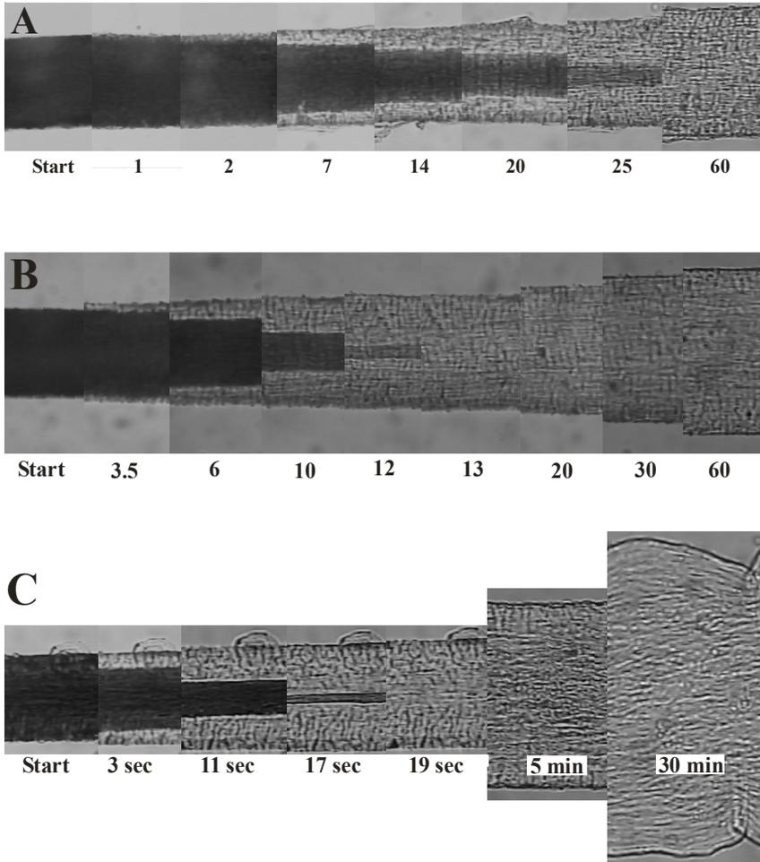
Fig. 67: Penetration of alkali into the hair fiber and swelling of the hair fiber at different pH. The same part of the fiber is always shown. Time is given in minutes, except for pH 13.4. There, the exact time is given for each picture.
