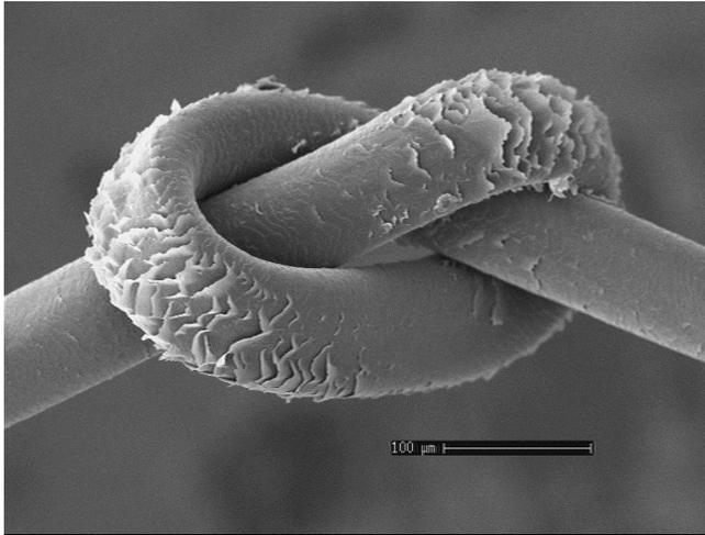
Fig. 23: Typical hair damage (“fir cone” effect) of an Caucasian hair induced by a strong PW or bleaching.
