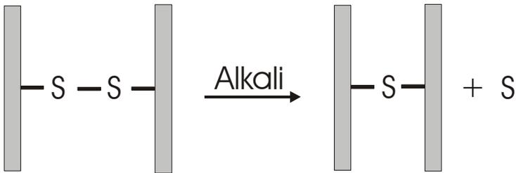
Fig. 12: Schematic diagram of the formation of lanthionine (monosulfide bridge) from CyS-SCy (disulfide bridge) during an alkaline treatment.
