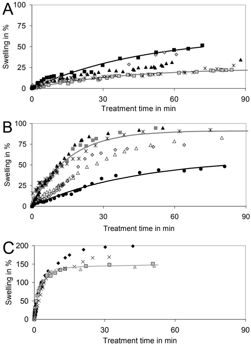
Fig. 64: Swelling of blond, Caucasian hair fibers when treated at different pHs. Each symbol shows a single experiment. Lines represent examples for fitted data by using eq. 3.25.
