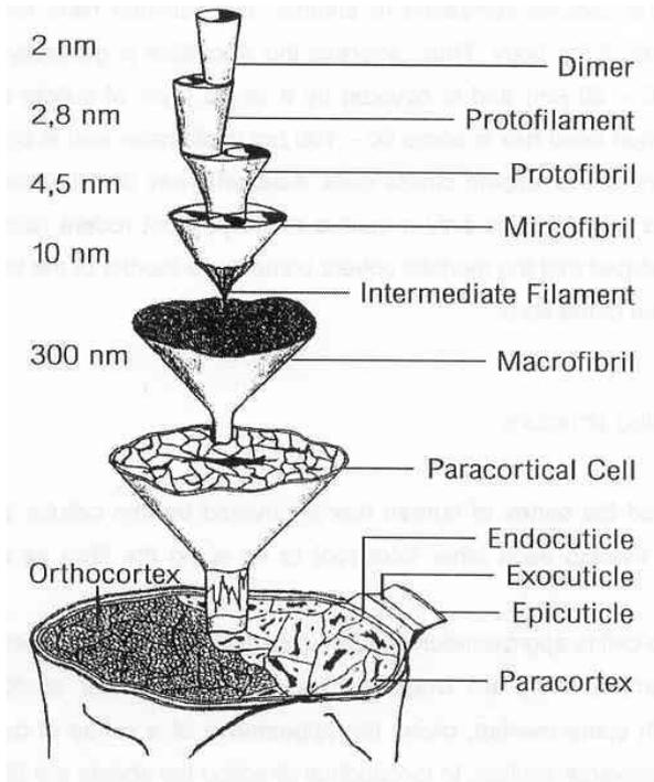
Fig. 1: Schematic diagram of the general structure of keratin fibers (here: wool); adapted from /2/.
