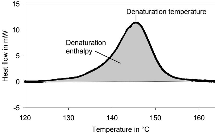
Fig. 35: HP-DSC diagram (black line) of relaxed Caucasian hair in water. The highest point of the black curve represents the denaturation temperature, the grey shaded area beneath the curve (integration of the heat flow curve over time) the denaturation enthalpy.
