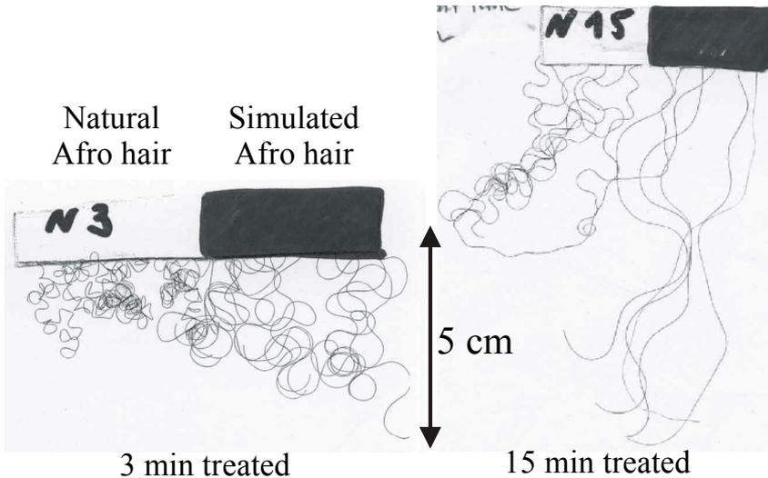
Fig. 41: Photos of simulated and natural Afro hair treated for 3 min and 15min, respectively, with NaOH.
