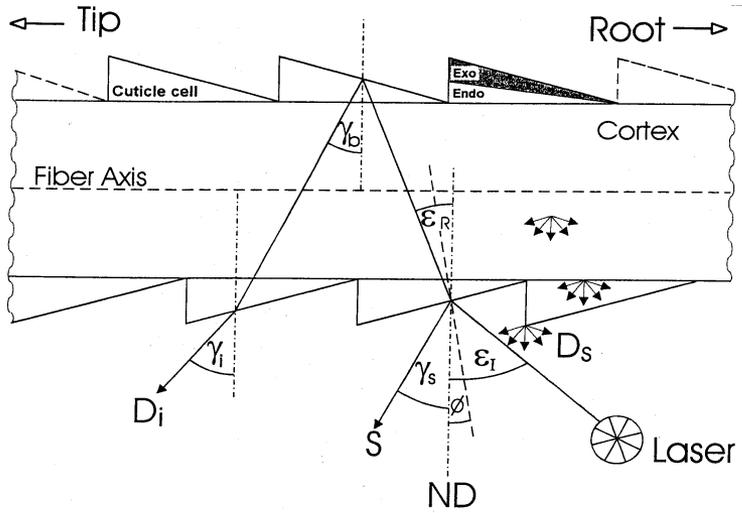
Fig. 26: Principles of light reflection and backward scattering on and in a hair fiber /34/.
