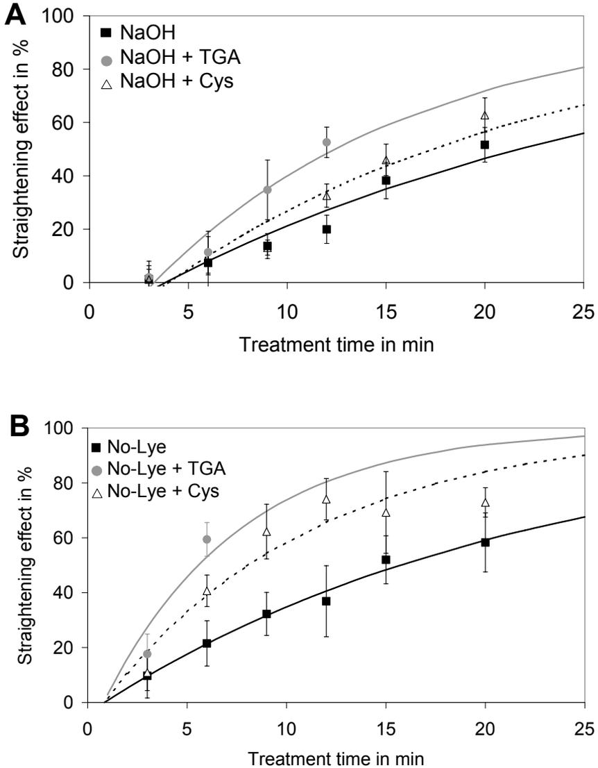
Fig. 43: Straightening effect (natural Afro hair) of different relaxer creams (with and without TGA or cysteine) versus relaxing time. The error bars represent the standard deviation ( $n = 8$ ).
