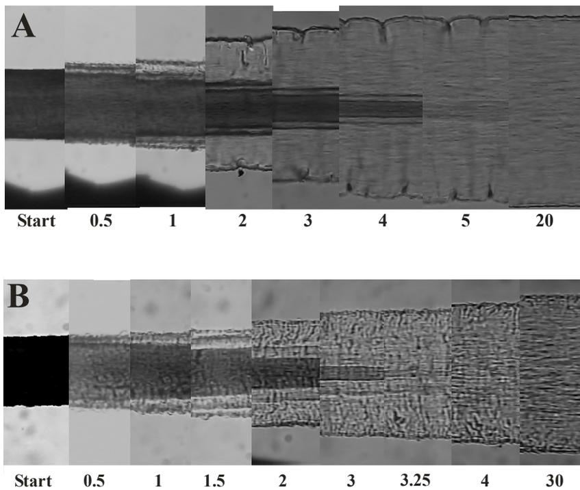
Fig. 68: Penetration of alkali and thioles into the hair fiber and swelling of the hair fiber at pH 12.8. The same part of the fiber is always shown. Time is given in minutes.
