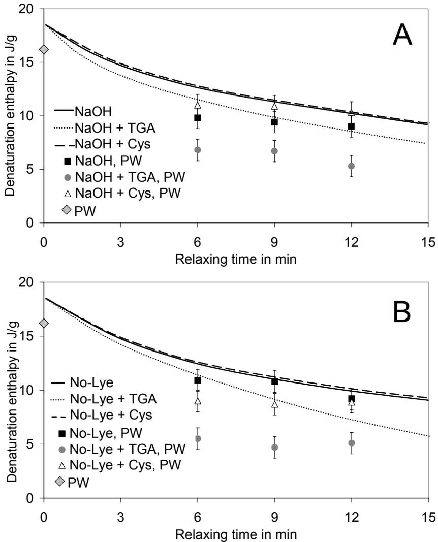
Fig. 60: Relationship between denaturation enthalpy of relaxed and subsequently permed hair and relaxing time. The curves represent the fitted values of enthalpy for the only relaxed hair; the dots are values for the relaxed and permed hair;  $\diamond$  = enthalpy of only permed hair. Error bars represent the standard deviation.
