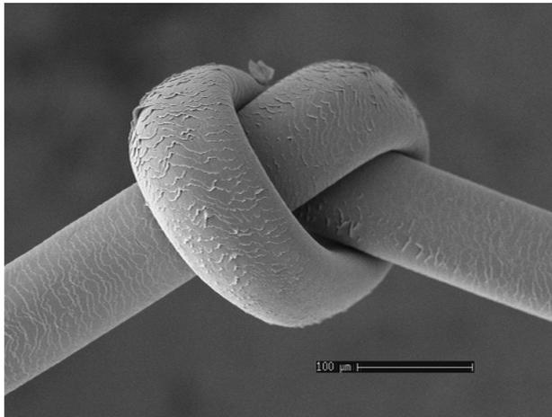
Fig. 22: Knot in an undamaged Caucasian hair in the SEM
