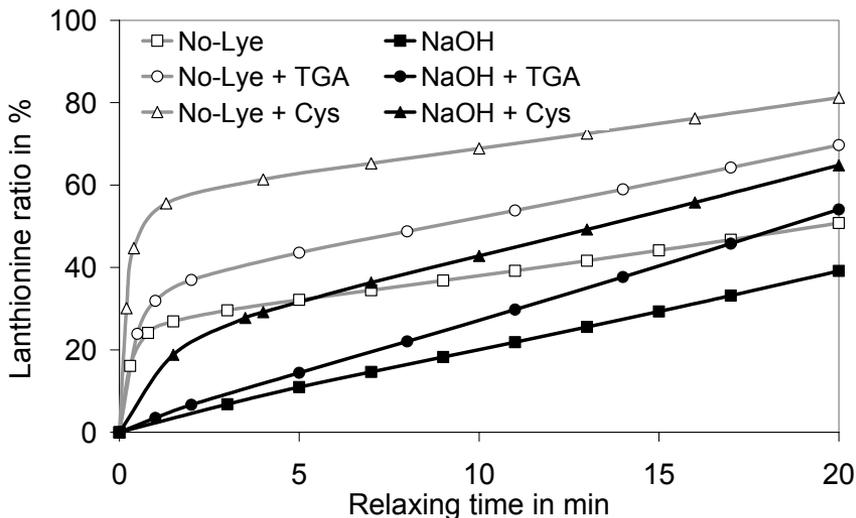
Fig. 49: Percentage of degraded cystine (by alkali) which is transformed into lanthionine (lanthionine ratio) versus relaxing time. The curves are calculated for different times by using eq. 3.8 and 3.9, and the values of Tab. 8 and 9.
