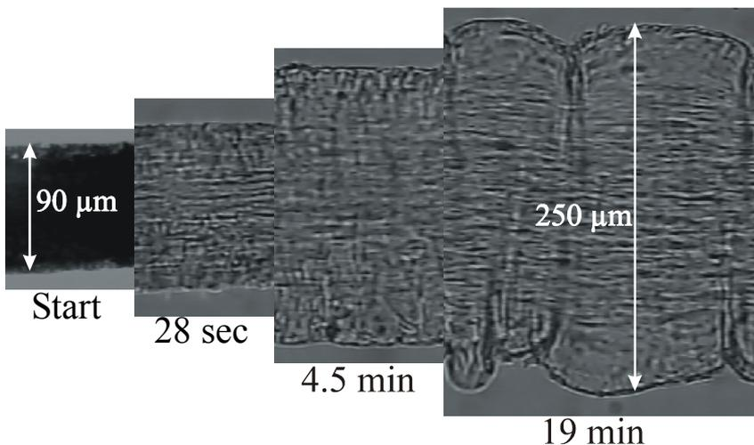
Fig. 63: Process of swelling of a blond, Caucasian hair fiber at pH 13.4. The pictures always show the same segment of the hair fiber for different treatment times.
