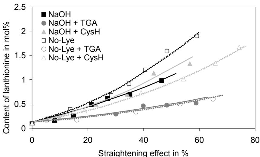
Fig. 50: Lanthionine content versus straightening effect. The values of Lan are measured data, and the values of straightening effect are recalculated using eq. 3.6 and parameters of Tab. 6.
