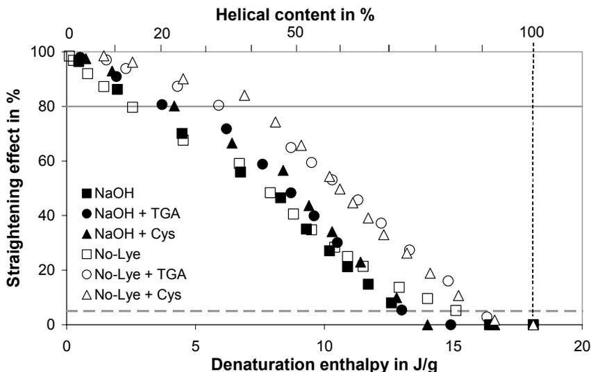
Fig. 53: Dependence of the straightening effect on the denaturation enthalpy.
