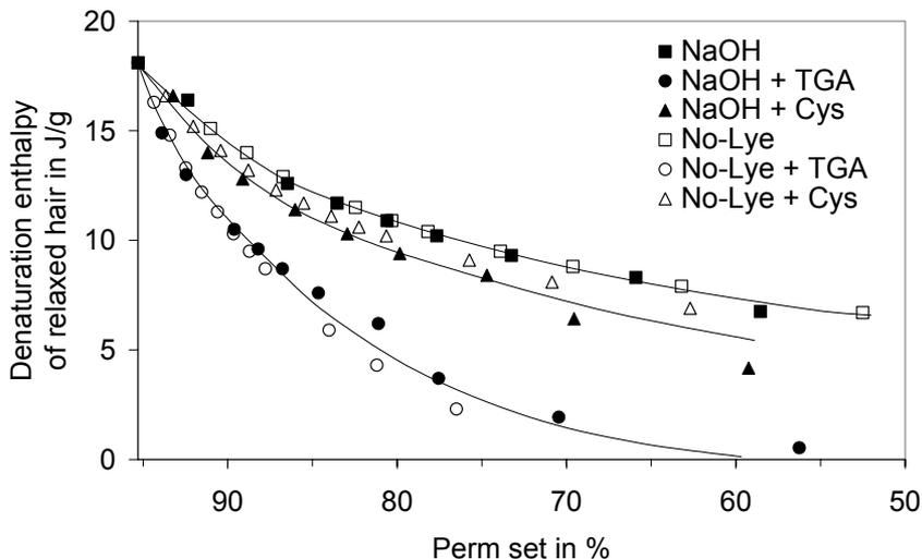
Fig. 62: Dependence of perm set on denaturation enthalpy. The data of perm set are calculated using eq. 3.16, the parameters are taken from Tab. 12. The data of denaturation enthalpy are measured data.
